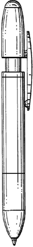
Figure 2. Example of a design for a horizontal break on a writing instrument.
